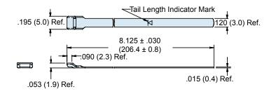
The 600-057 Micro Band is precision constructed of 300 Series SST/Passivate, and designed for use with the 600-061 Hand Banding Tool or the 600-068 Pneumatic Banding Tool. Double-wrapped bands will accommodate diameters up to approximately .88 inches (22.4). Bands may be ordered flat (600-057), or precoiled (600-057-1). Bands come bagged and tagged in quantities from 1 to 100.
