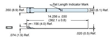
The 600-052 Standard Band is precision constructed of 300 Series SST/Passivate and designed for use with the 600-058 Hand Banding Tool or the 600-067 Pneumatic Banding Tool. Double-wrapped bands will accommodate diameters up to approximately 1.8 inches (45.7). Bands may be ordered flat (600-052) or precoiled (600-052-1). Bands come bagged and tagged in quantities from 1 to 100.
